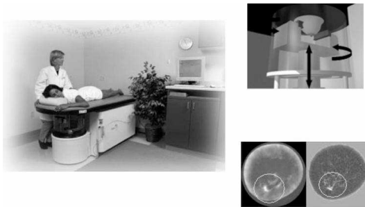
Figure 8: Ultrasound scanner developed by TechniScan, Salt Lake City (left), scanning geometry (top right) and reconstruction of speed of sound and attenuation (bottom right).
